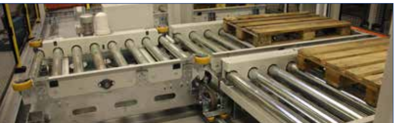
Only one drive to an unlimited number of roller conveyors
